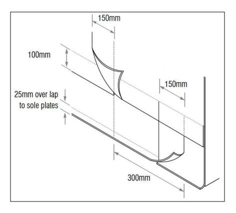
Figure 3: Drawing indicating fixing frequency in factory/on site
