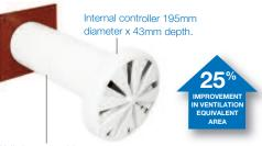
Wall sleeve outside diameter 99mm. Suitable for any wall thickness up to 350mm as standard (or more to special order). Please note: 100-110mm diameter core bit required for fitting.
