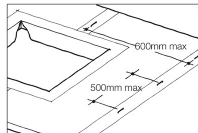
4. Secure membrane to sheathing with austenitic stainless steel staples at 500mm centres vertically and 600mm horizontally
