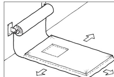
2. Pull membrane taut over panel with reflective surface uppermost (facing into cavity)
