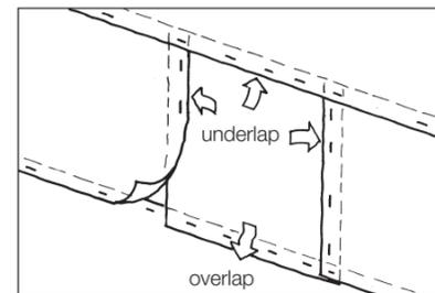
2. Secure membrane to sheathing with austenitic stainless steel staples at 500mm centres vertically and 600mm horizontally
