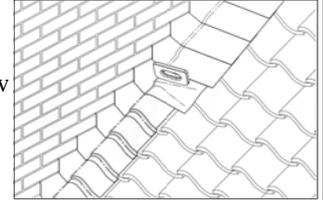
If the flashings are to be left unsecured for any length of time or are subject to strong winds, it is advised that a batten be fixed across the face of the flashing to prevent wind uplift.
