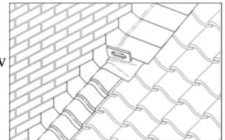
If the flashings are to be left unsecured for any length of time or are subject to strong winds, it is advised that a batten be fixed across the face of the flashing to prevent wind uplift.
