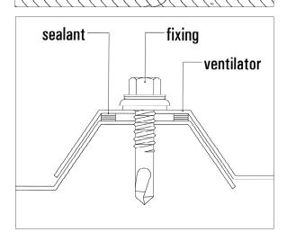
Locate the position of the ventilator centrally between two supports and mark the outline.
