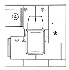
4. It may be easier to locate and fit the upper forming before placing this tile\* in position. Hold the upper forming up the roof slope, slide it down, engaging the clip (or clips) on the underside to the lower forming.
