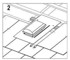
**NOTE:** Ensure the ventilator is not directly above a rafter and the batten cantilever is not excessive.
