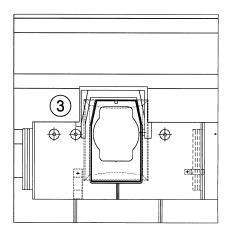
**3.** Place the lower forming in position, ensure all clips locate under the adjacent tiles at side and lower edge, nail in position.
