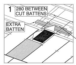
1. Lay slates to the required position of the ventilator. Cut the slate directly below the ventilator so that it does not protrude past the slate batten. Cut a 280mm wide gap in the batten at the head of the slate as shown.
