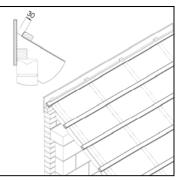
Lay the underlay in the normal way, but 2. ensure that any fixings are set back at least 30mm from the inside face of the ridge board and there is sufficient free edge on the underlay to enable it to be wrapped onto the top batten.
