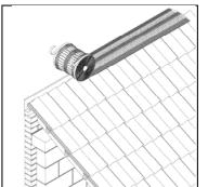
3. Unroll the Protect Fulmetal Rediroll over the ridge board ensuring a 75mm overlap onto the tip course of tiles. Secure in place onto the ridge board every 300mm with clout nails or staples. Any joins should be overlapped by a minimum of 75mm
