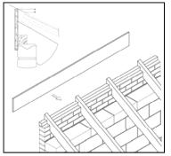
1. Fix a suitably sized ridge board to the end of the rafters. Check that the top of the board will be above the uppermost point of the finished height the top course of tiles. of
