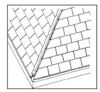
3. Screw fix hip batten constructed from 50 x 50mm timber to the supports. Complete tiling, cutting the tiles neatly against the hip batten. No cut tiles should be more than 30mm from the hip batten. Small tile cuts should be secured mechanically or by using a proprietary adhesive or other fixing method.
