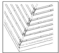
2. Hip batten supports in 50mm x 50mm timber should be screw fixed at the eaves and apex and spaced along the line of the hip rafter in between the tiling batten spaces as shown. Supports could be constructed from 2 x 25mm tiling battens.
