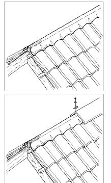
4. Unroll the Protect Fulmetal Rediroll centrally over the ridge batten ensuring a 75mm overlap on each side of the top course of tiles. Secure in place every 300mm with clout nails or staples. Any joins should be overlapped by a minimum of 75mm.
