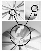
4 Once in place, locate the fascia over the base unit ensuring that the placement lug of the back plate (a) lines up with the receptor void on the perimeter of the fascia (b).
