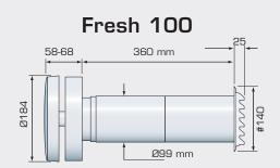
Maximum wall thickness 360 mm (standard). Hole-punching Ø102 mm
