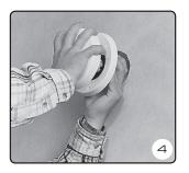
Open the front cover. Press the cover inwards and turn it clockwise. Remove the filter holder and filter.
