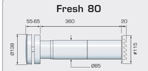
Maximum wall thickness 360 mm (standard). Hole-punching Ø86 mm.
