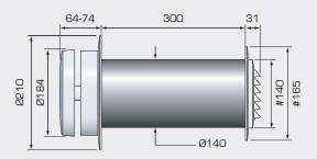
Maximum wall thickness 300mm (standard). Hole-punching Ø150mm. Internal cover plate #210 as standard.
