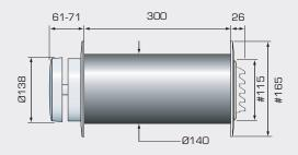
Maximum wall thickness 300mm (standard). Hole-punching Ø150mm. Internal cover plate #165 as standard.
