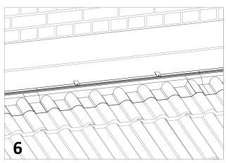
6. Bring down the flashing from the wall on to the top face of the AV50, terminating it behind the ridge of the forming above the ventilation holes. Tuck the flashing behind the clips to help prevent uplift. Also ensure that the wall flashing covers the open ends of the vent in order to prevent both weather and insect ingress.
