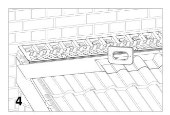
4. Moving back to the AV50 installed first, ensure that the roof covering under the flashing is clean, dry and dust free. Remove the release liner from the back of the AluFlash apron. Using an AluFlash dressing tool, dress the flashing onto the tiles to achieve a weatherproof junction. Trim away any excess flashing on the left hand side which overhangs the tile.
