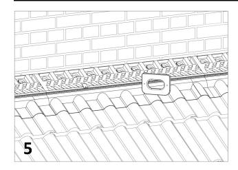
5. Continue to work along the roof, dressing the flashing to the tiles in the same manner as above. Always ensure the surface is clean, dry and dust free to ensure a bond is generated between the apron and roof covering.
