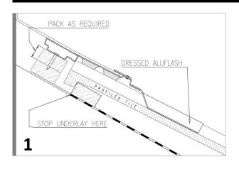
1. Before installation of the vent, check that a suitable air gap and supporting batten for the AV50 is present between the top course of tiles and wall. Depending on the tile type, additional packing may be required to support and fix the AV50 to.
