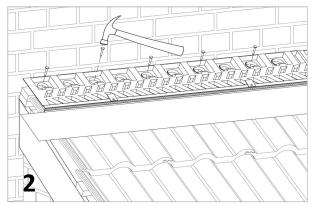
2. Starting on the left hand side of the roof, position the first AV50 so that its left hand edge is level with the edge of the tile. Check that the vent is parallel to the wall and the plastic part of the AV50 sits on the tile as illustrated in the section view in stage 1 above. Fix the AV50 in place as shown.
