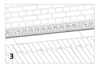
3. Moving from left to right, continue to install the AV50 vents along the roof/abutment ensuring that the plastic and flashing of adjacent AV50s overlap one another. Cut the final AV50 to length level with the edge of the last tile, whilst ensuring sufficient flashing is retained to dress over the full width of the tile.
