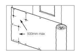
2. Secure membrane with austenitic stainless steel staples
