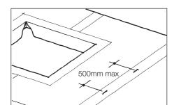
4. Secure membrane to sheathing with austenitic stainless steel staples, ensuring laps are taped
