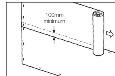
4. Fix second layer ensuring all laps are taped and repeat up to roof abutment
