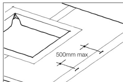
4. Secure membrane to sheathing with austenitic stainless steel staples, ensuring laps are taped
