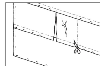
6. Replace damaged and torn membrane
