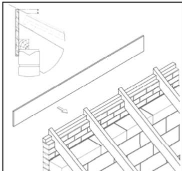
1. Fix a suitably sized ridge board to the end of the rafters. Check that the top of the board will be above the uppermost point of the finished height of the top course of tiles.
