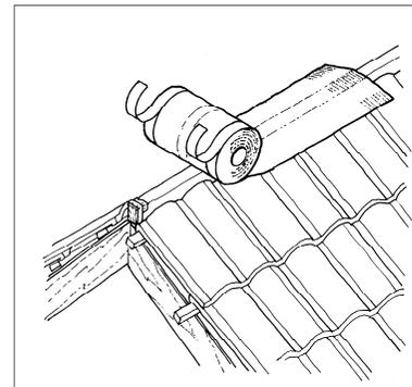
4. Unroll the Protect Fulmetal Rediroll centrally over the ridge batten ensuring a 75mm overlap on each side of the top course of tiles. Secure in place every 300mm with clout nails or staples. Any joins should be overlapped by a minimum of 75mm.
