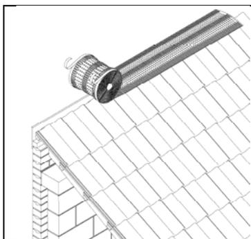
3. Unroll the Protect Fulmetal Rediroll over the ridge board ensuring a 75mm overlap onto the top course of tiles. Secure in place onto the ridge board every 300mm with clout nails or staples. Any joints should be overlapped by a minimum of 75mm
