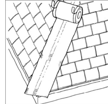
4. Working from the eaves, secure the Protect Fulmetal Rediroll in place centrally over the hip batten using corrosion resistant nails or staples. Roll out along the hip batten and fix at 300mm centres. Remove protective paper from the adhesive strip and press down firmly onto dry, clean tiles all the way up both sides of the hip. A hip carrier is available to assist with aligning the hip tiles when used with profiled tiles if required (available to separate order)
