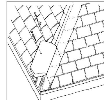
5. Using a 100mm screw provided secure the block end hip tile to the hip batten. (it may be necessary to drill a hole in the hip tile approximately 30-40mm from the block end for this purpose.) Fix hip tiles up to the apex using the 100mm screws and fixing plates provided. An optional screw sleeve is included if the user perceives that there may be a risk of light bleed between hip tiles.
