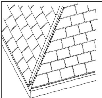
3. Screw fix hip batten constructed from 50 x 50mm timber to the supports. Complete tiling, cutting the tiles neatly against the hip batten. No cut tiles should be more than 30mm from the hip batten. Small tile cuts should be secured mechanically or by using a proprietary adhesive or other fixing method.
