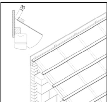
2. Lay the underlay in the normal way, but ensure that any fixings are set back at least 30mm from the inside face of the ridge board and there is sufficient free edge on the underlay to enable it to be wrapped onto the top batten.
