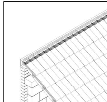
4. Remove the protective paper from the adhesive strip and press down firmly onto dry, clean tiles all the way along the ridge. For deeply profiled tiles, additional care is needed to work the Fulmetal Rediroll into the pans.
