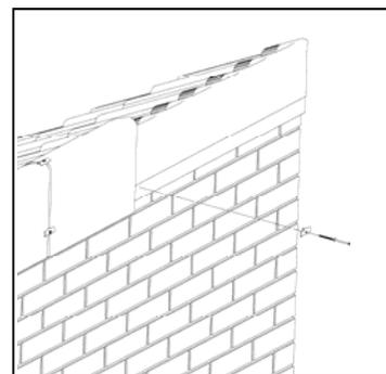
6. Secure the vertical face of the ridge tiles into the ridge board and into the wall plate timber with further fixing plates and screws.
