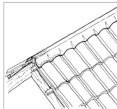
5. Remove protective paper from the adhesive strip and press down firmly onto dry, clean tiles all the way along the ridge. For deeply profiled tiles, additional care is needed to work the Fulmetal RediRoll into the pans.
