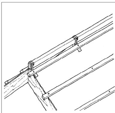
3. Fix the top tiling batten ensuring an air gap is maintained.
