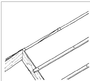
1. For unventilated dry ridge applications, install the underlay as normal.
