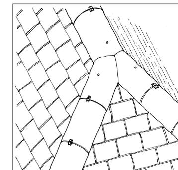
6. At the apex close mitre the hip and ridge tiles, drill and secure to the hip and ridge batten using the 100mm screws provided. If Protect Fulmetal Rediroll is not used on the ridge continue the roll 200mm onto the ridge in place of the standard lead saddle detail.
