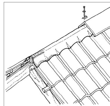
6. Locate the block end ridge tile over the centre of the roll and secure it with a screw (it may be necessary to drill a hole in the ridge approximately 30-40mm from the block end for this purpose.) Continue along the ridge fixing each ridge tile with the plates and screws provided. An optional screw sleeve is included if the user perceives that there may be a risk of light bleed between ridge tiles.
