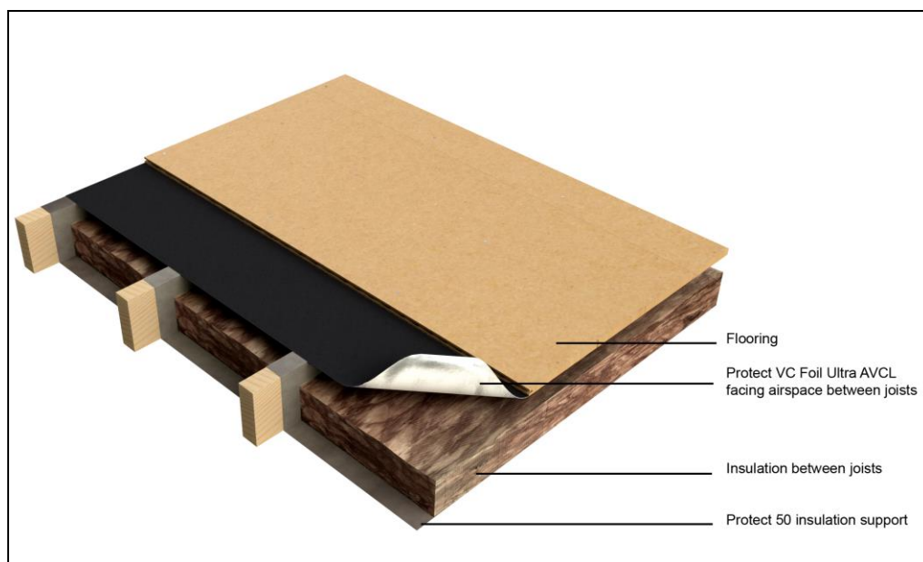
Figure 3: Suspended Timber Floor Construction
