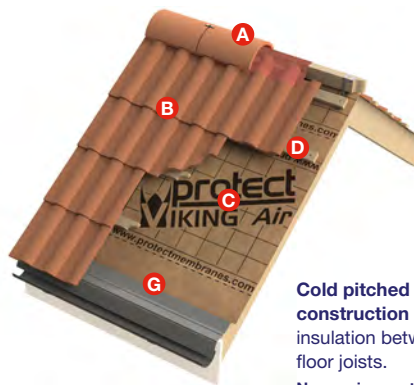
Cold pitched roof construction with roofing underlay installed on sarking board. See table below for ventilation requirements.
